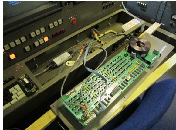
Trackerball and E.C.'s keyboard Removed and inverted for fault finding
