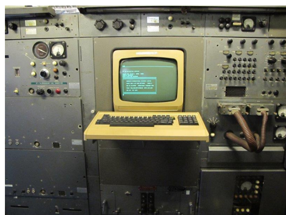
FT81 - Correct Display Refitted to L Rack in the LCP
