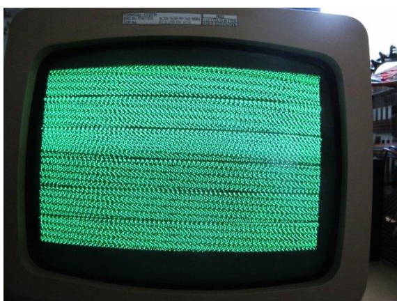
FT81 - Faulty Display Not exactly readable!
