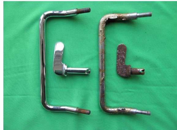
Comparing the refurbished and original chrome handles Before and after
