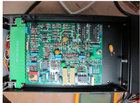
Power Supply G15-16S – Control Card Bead tantalum capacitors also changed as a matter of course when a fault develops on the control card
